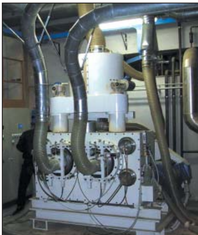
Pelletisation machine ETS® (ECOTRE System)
