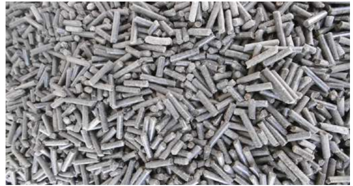
Dried pelletized sewage sludge used as feedstock to produce green diesel and green gasoline.
