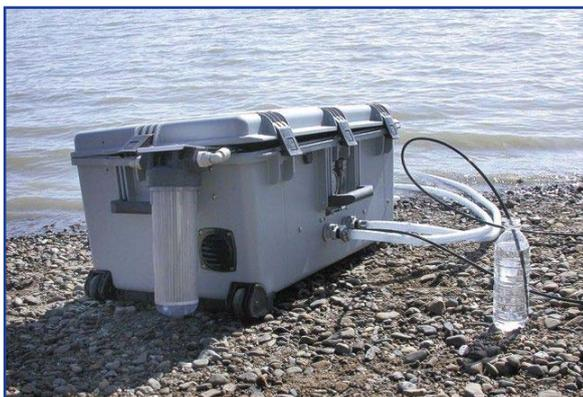
Portable seawater RO system Aquifer from Spectra Watermakers with daily production up to 680l of freshwater.
