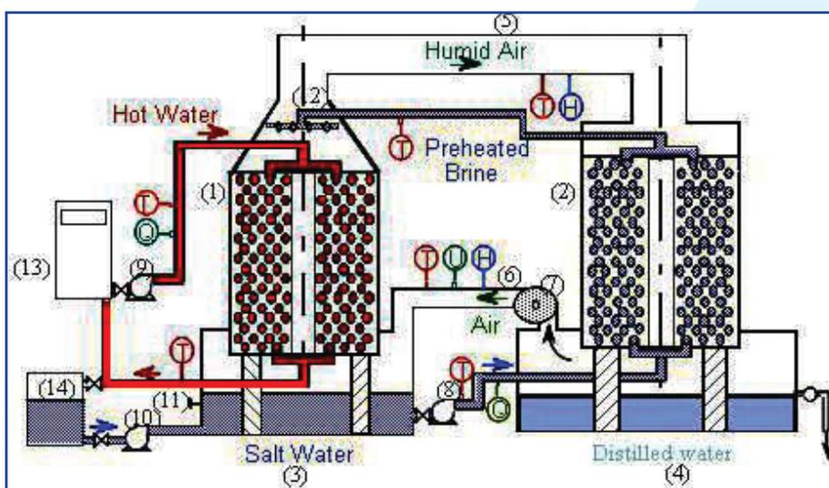
Figure 1: Presentation of the desalination prototype functioning by the aero-evaporo-condensation process (A.E.C.P).
