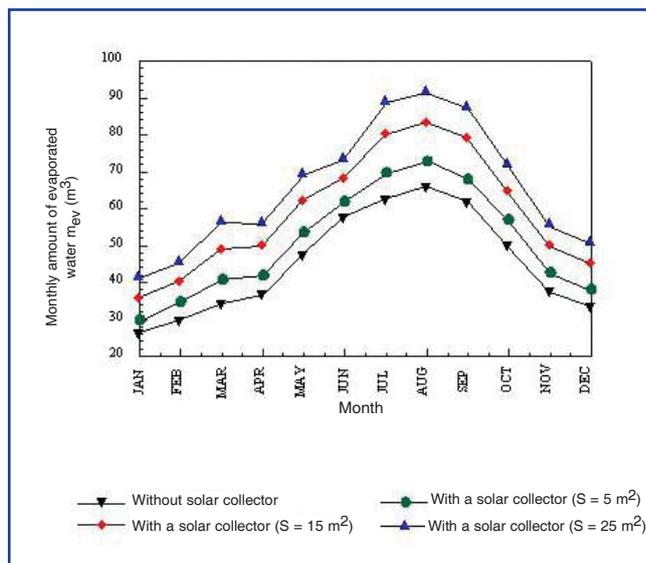
Figure 2: Variation of the monthly amount of evaporated produced by AEC for different solar collector surfaces ( $m_{air} = 0.3 \text{ kg/s}$ ), Bourouni et al 2003.
